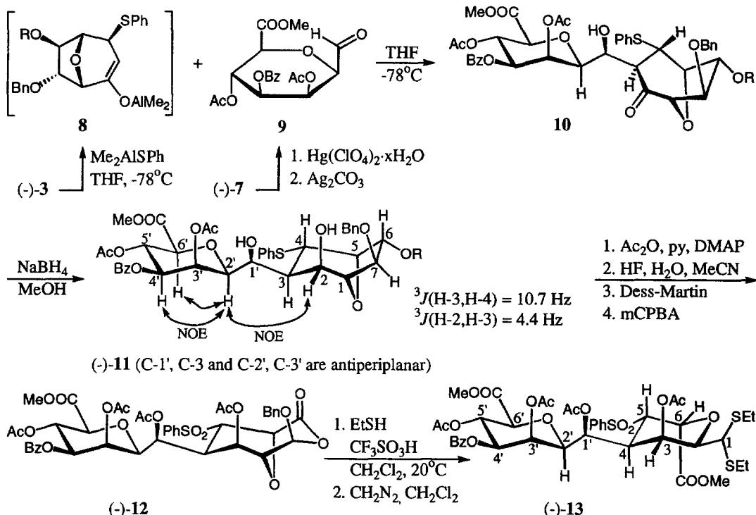
Hydrolysis of the dithioacetal (-)-7 (Hg(ClO<sub>4</sub>)<sub>2</sub>·xH<sub>2</sub>O, MeCN, 20°C, then: Ag<sub>2</sub>CO<sub>3</sub>, MeCN/CHCl<sub>3</sub>, 20°C) liberated the unstable aldehyde 9 which was reacted with the aluminum enolate 8 generated by addition of Me<sub>2</sub>AlSPh<sup>17</sup> to enone (-)-3. Out of four possible diastereomeric aldols only 10 was formed. Because of its
